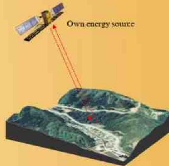
As **passive** microwave sensors deal with very low resolution, more applications in these wavelengths use **active** sensors
