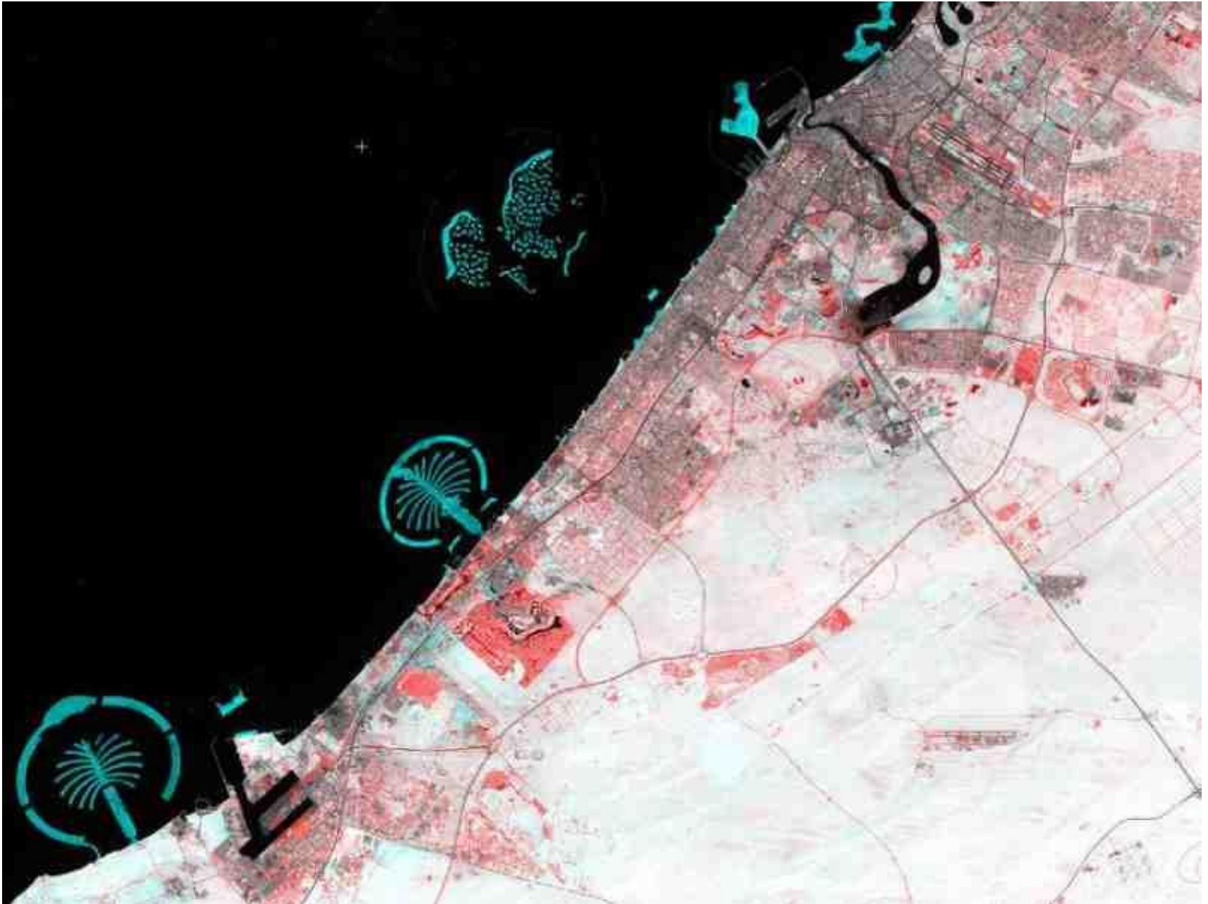
Simultaneous display band 3 for 2000 (red) and 2006 (blue-green) - Dubai
