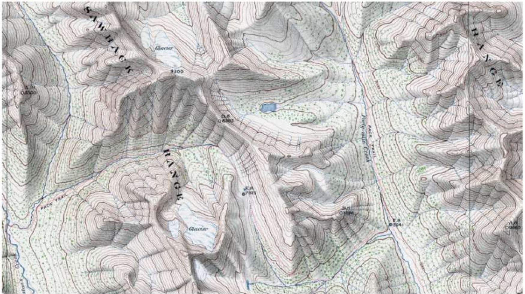
Figure 3: Forty-Mile Creek 1890. Topographical Surveys Branch, Department of the Interior, Ottawa. Triangulation by W.S. Drewry, D.L.S. Topography by J.J. McArthur, D.L.S. 1:40,000
