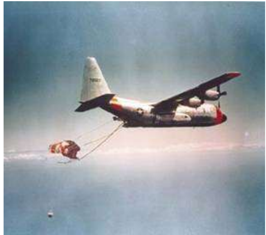
A JC-130 recovery aircraft of the U.S. Air Force retrieves a Corona satellite film-return capsule, also known as a "bucket," over the Pacific Ocean. Photo credit: CSNR collection.
