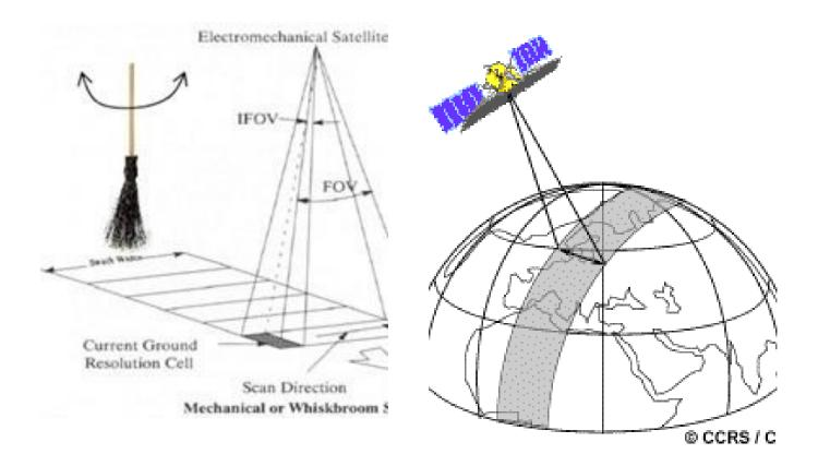
**a. Whiskbroom** (mirror/ crosstrack): a small number of sensitive diodes for each band sweep perpendicular to the path or swath, centred directly under the platform, i.e. at 'nadir' e.g. LANDSAT MSS /TM/ETM
