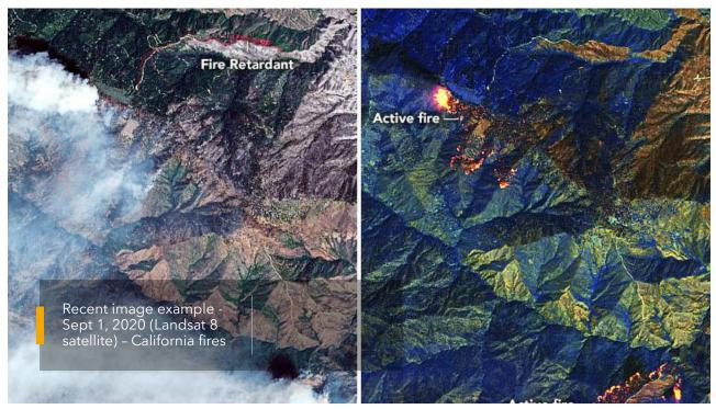
**Myth #1 about remote sensing:** This is a satellite photograph, but most are NOT e.g. the previous slide image (the fires) was produced from a scanner, not a camera
