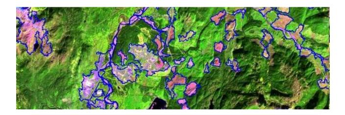
Digital remote sensing imagery -- autogeneration of vector layers (polygon data)
