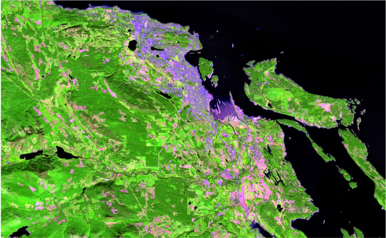
Fig. 2 Landsat 8 image of the city of Nanaimo, BC from September 2, 2014. The image is displayed using bands 456 (Red, Near-Infrared, Mid-Infrared respectively).
