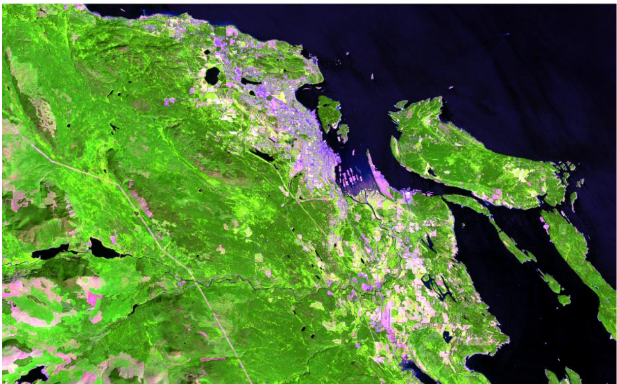
Fig. 1 Landsat 5 image of the city of Nanaimo, BC from August 8, 1986. The image is displayed using band 345 (Red, Near Infrared, and Mid-Infrared respectively)
