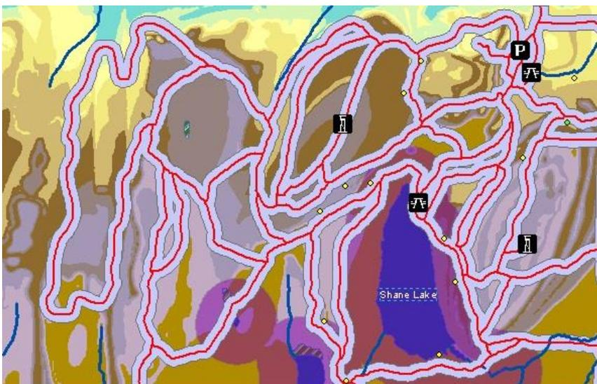
Figure 3. Contours used to generate a elevation raster showing changes in elevation based on the contour lines joining regions of elevation with a 20m buffer set around trails and a 100m buffer set around the lakes.
