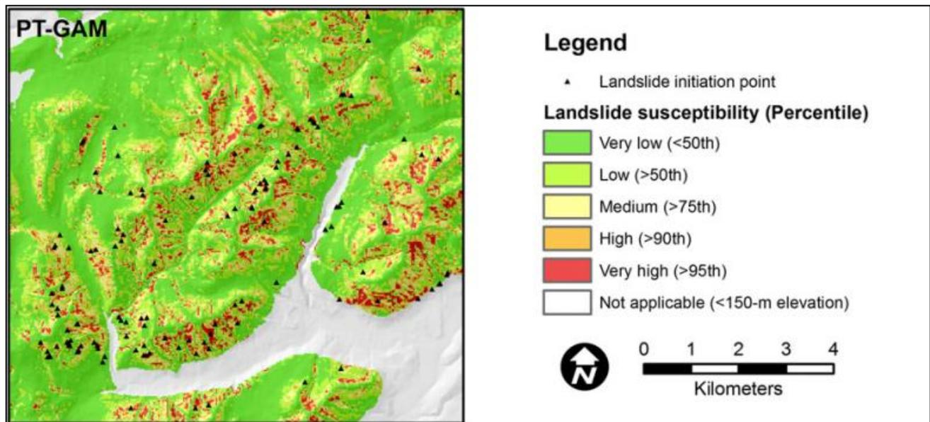
Figure 7 Landslide hazard map showing areas along the Klanawa River Watershed that are susceptible to landslides (Source: Goetz et al. 2011)
